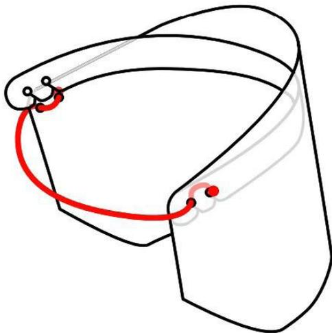
Once assembled, your finished face shield, using elastic, should look like this. (The string version ties in the back.)
